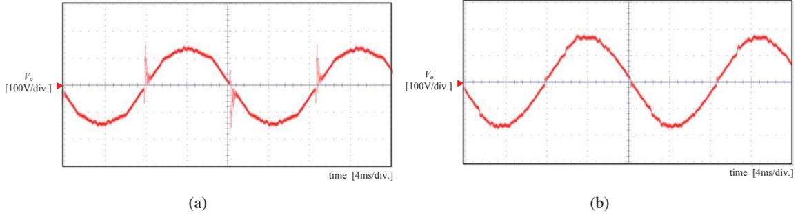
Figure 7: Experimental waveforms of output voltage. (a) When the equivalent controller is used. (b) When the proposed ISMC is used.
