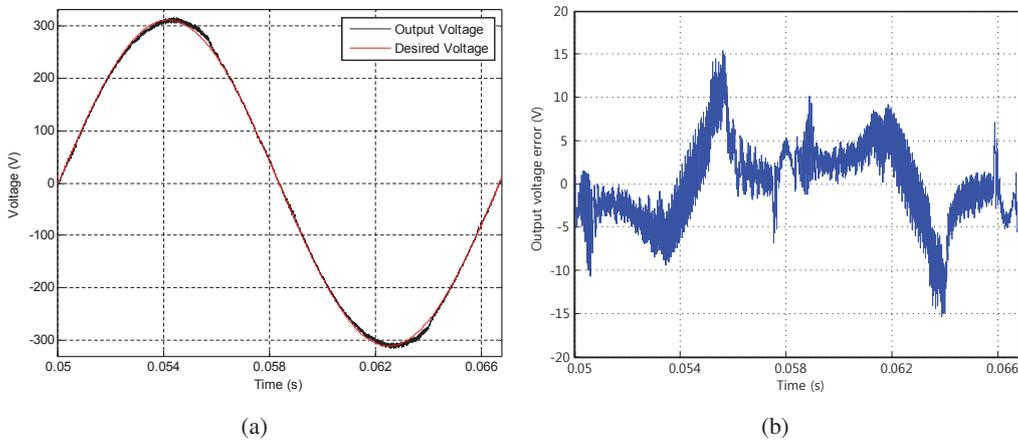
Figure 5: Simulation results with the proposed ISMC when the input voltage is 50 V. (a) Output voltage waveform. (b) Output voltage error.
