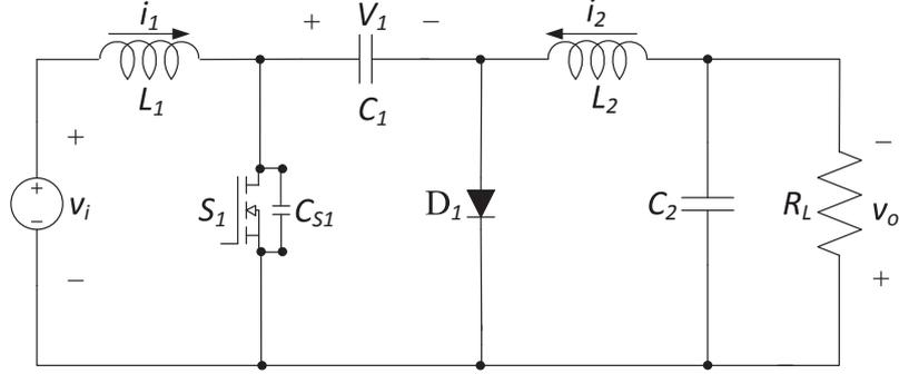
Figure 2: The equivalent circuit of Cuk inverter.
