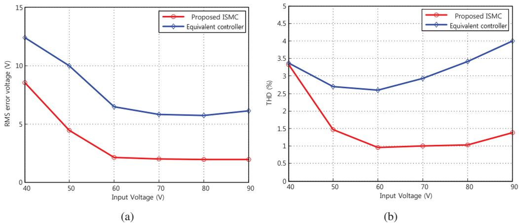
Figure 6: Simulation results as the input voltage varies from 40 V to 90 V. (a) RMS of output voltage error. (b) THD.
