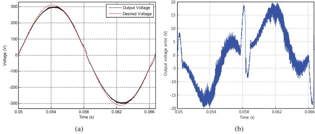
Figure 4: Simulation results with the equivalent controller under the input voltage is 50 V. (a) Output voltage waveform. (b) Output voltage error.
