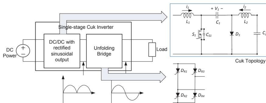
Figure 1: The circuit diagram of single-stage Cuk inverter.
