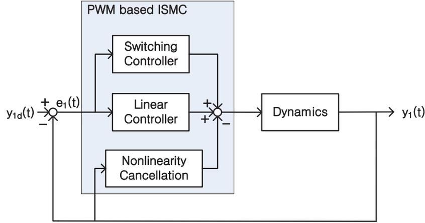
Figure 3: The schematic diagram of control system for the Cuk inverter.
