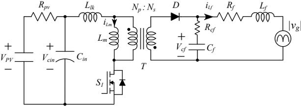
Fig. 2. The second-order model of the flyback converter.
