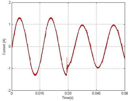
Fig. 12. Waveforms of the output current (red) and the desired output current (blue) when the output power is varied.
