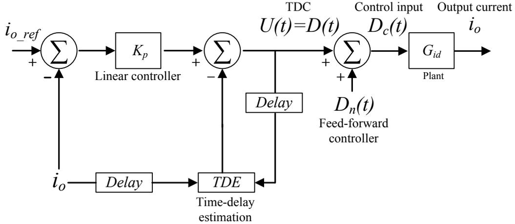
Fig. 3. The schematic diagram of the proposed controller.  $G_{id}$  is the control-input to output-current transfer function.
