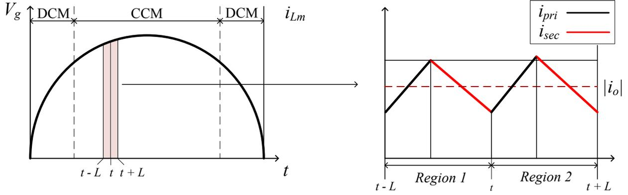
Fig. 4. The waveform of the magnetizing current in a single period in CCM.
