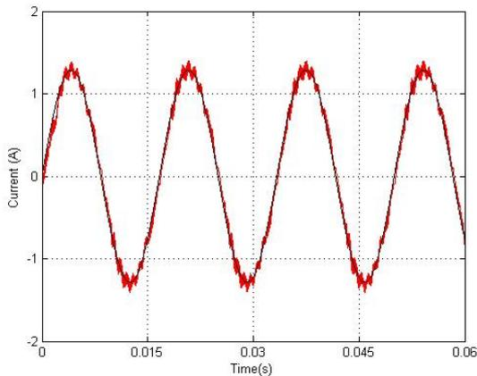
Fig. 9. Waveforms of the output current (red) and the desired output current (blue) when the feedforward and linear controllers are used.
