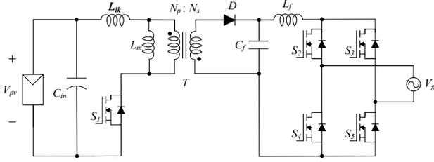
Fig. 1. The schematic diagram of the flyback converter.
