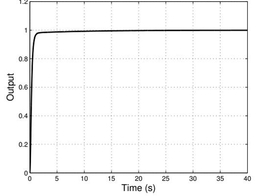
Fig. 6: Unit step response of the unstable plant with the TSK fuzzy PI controller.
