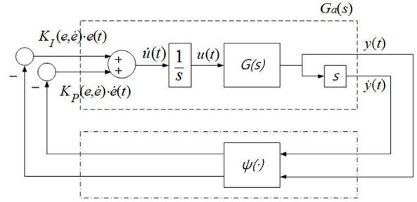
Fig. 4: Structure of the rearranged TSK fuzzy PI control system.
