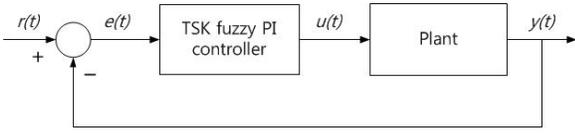
Fig. 1: Structure of the TSK fuzzy PI control system.
