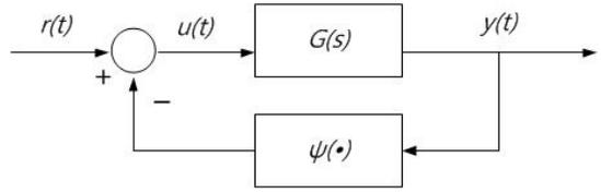
Fig. 2: Feedback connection which consists of linear dynamic system and sector-bounded nonlinearity .
