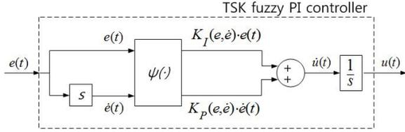
Fig. 3: Structure of the TSK fuzzy PI controller.
