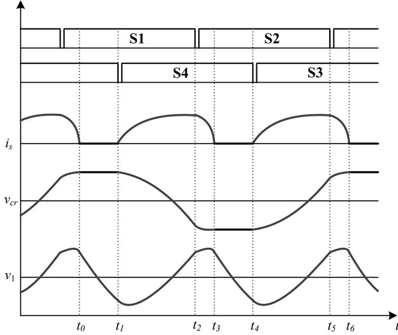
Figure 2: Simplified waveforms of  $i_s$ ,  $v_{cr}$  and  $v_1$
