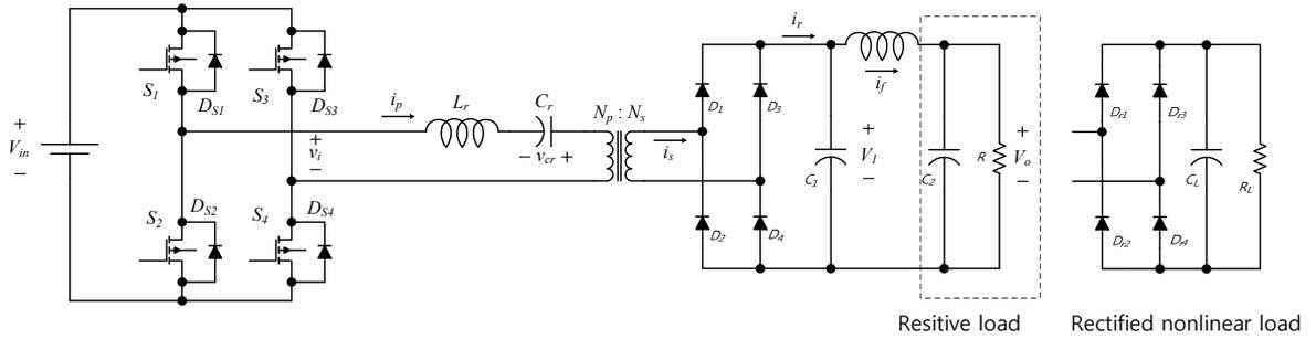
Figure 1: The circuit diagram of the PSFB-SRC.
