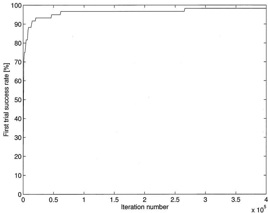
Fig. 10. First trial success rate of the current predictor trained with only the original samples.
