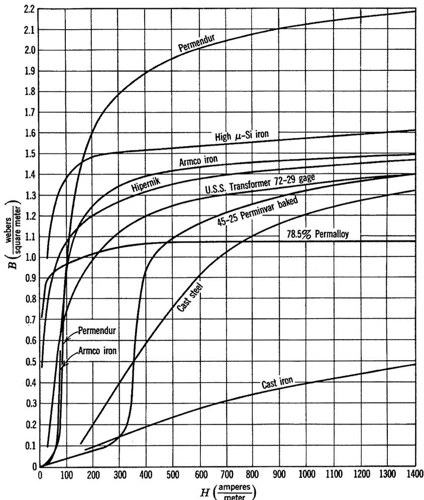
Fig. 2. Magnetization curves for several magnetic materials.
