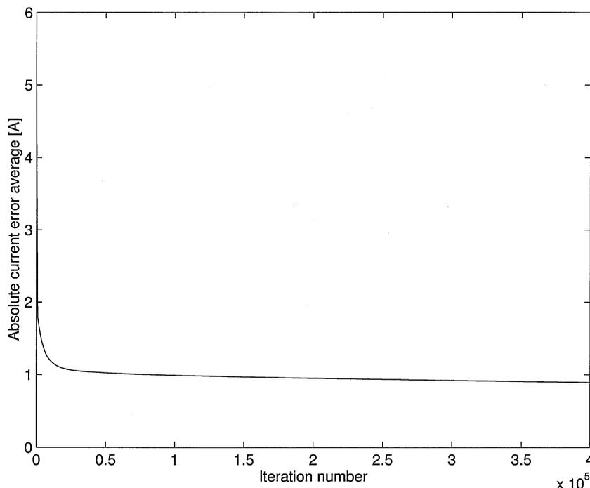
Fig. 9. Absolute current error average of the current predictor trained with only the original samples.
