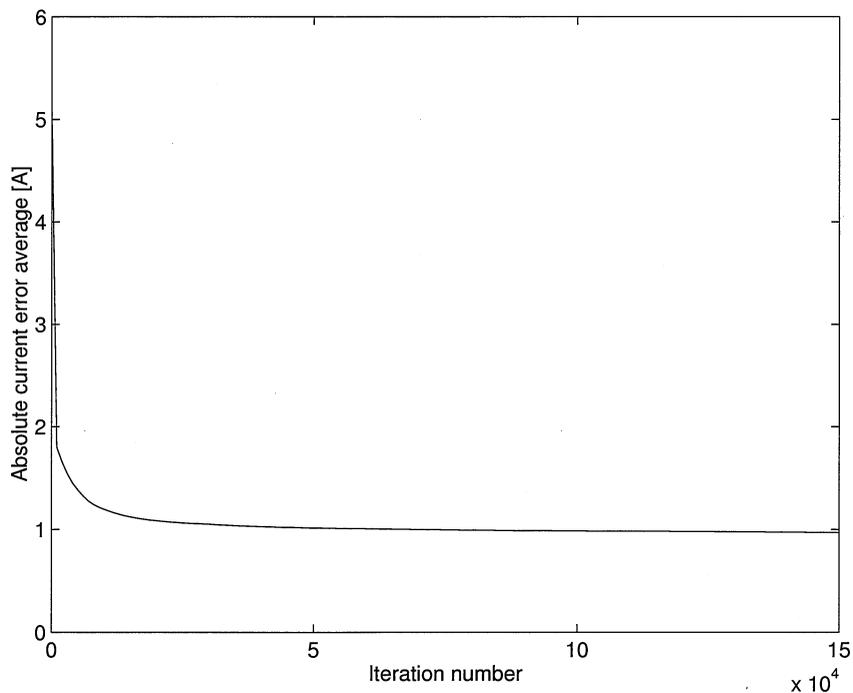
Fig. 11. Absolute current error average of the current predictor trained with the original plus the on-line samples.
