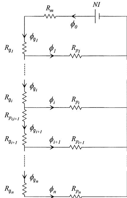
Fig. 4. Equivalent magnetic circuit of Fig. 3.
