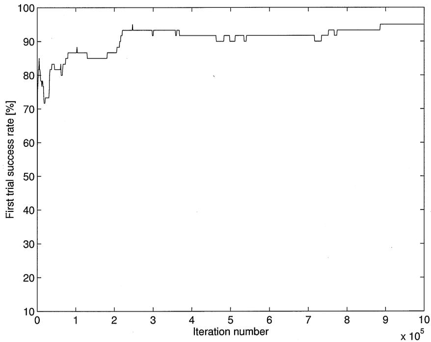
Fig. 16. First trial success rate of the current predictor trained with only the on-line samples.
