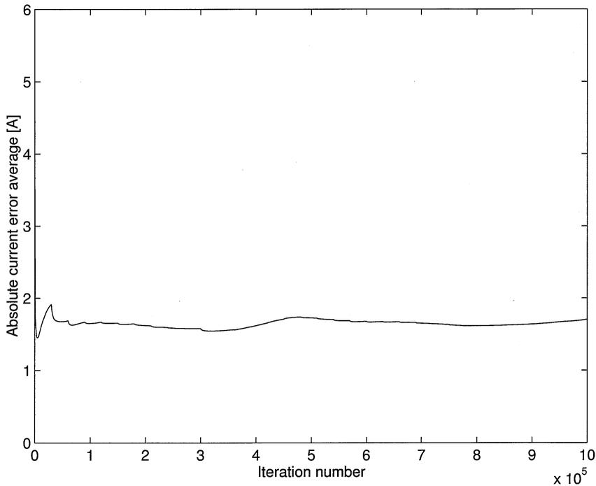
Fig. 15. Absolute current error average of the current predictor trained with only the on-line samples.
