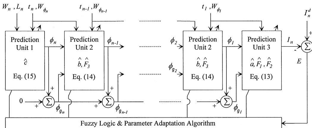
Fig. 5. The structure of adaptive fuzzy minimum current predictor.
