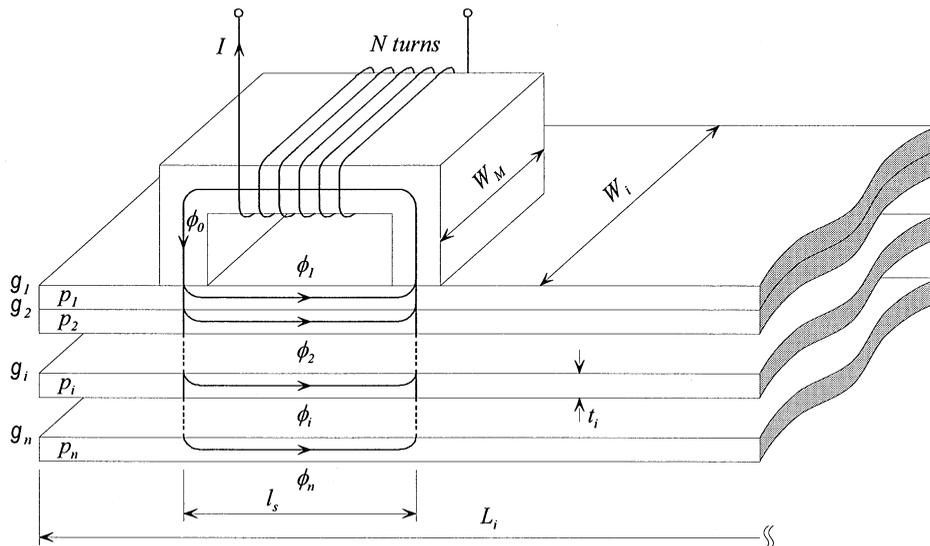
Fig. 3. Flux path of the magnet and steel plates.
