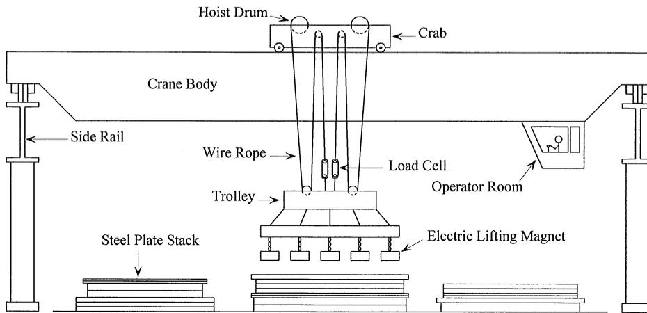
Fig. 1. The overview of overhead magnet crane.
