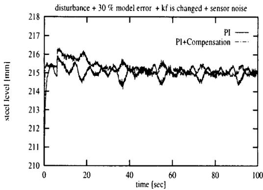
Fig. 12. Simulation with disturbance + 30% model errors +  $k_f$  change + sensor noise
