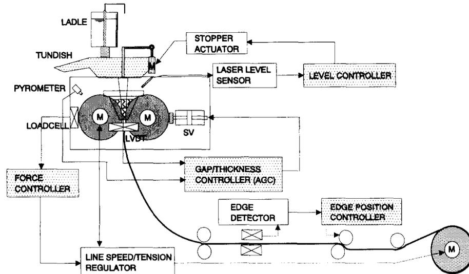
Fig. 1. Schematic layout of strip-caster pilot plant constructed in POSCO
