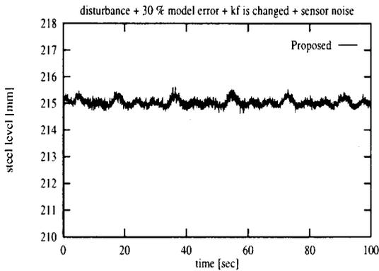
Fig. 13. Simulation with disturbance + 30% model errors +  $k_f$  change + sensor noise
