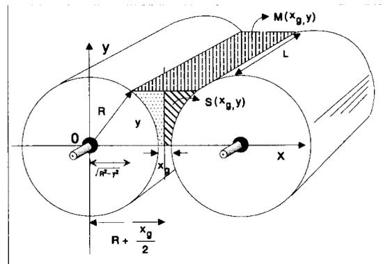
Fig. 3. Volume of molten steel filled between the twin roll cylinders.
