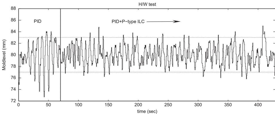
Fig. 12. Mold level when PID and PID + P-type ILC controllers are used.
