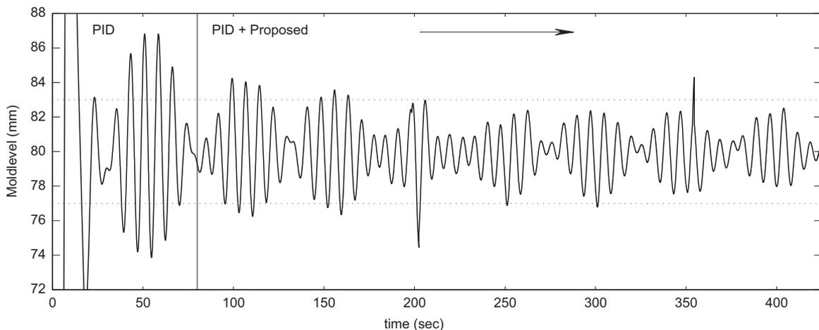
Fig. 8. Simulation result of the PID and proposed control system.
