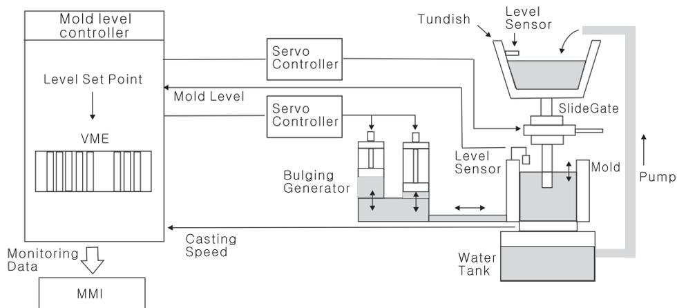
Fig. 10. Configuration of the proposed control system.
