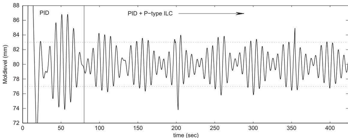
Fig. 7. Simulation result of the PID and P-type ILC control system.
