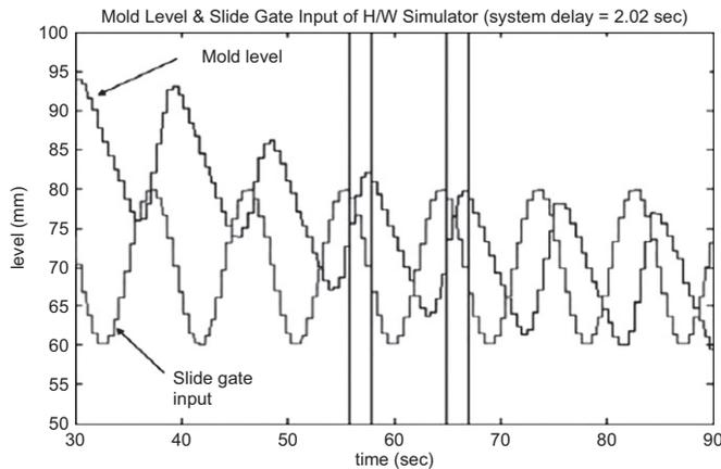
Fig. 6. System delay measurement.
