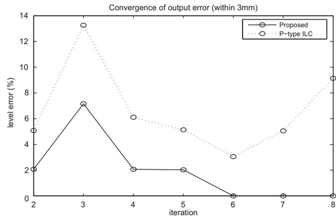
**Fig. 14.** The percentage of mold level error whose magnitude is  $\geq 3$  mm.
