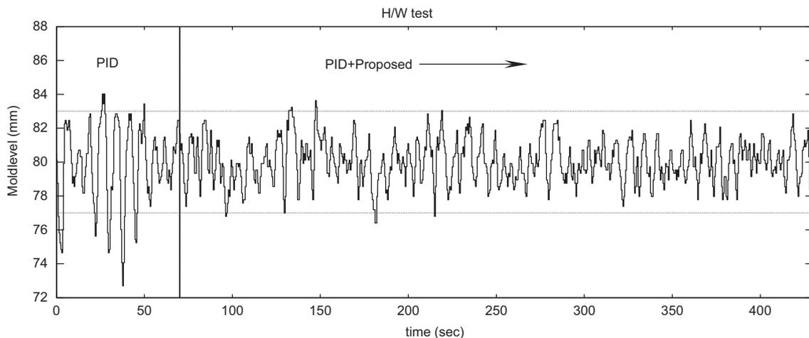
Fig. 13. Mold level when PID and PID + Proposed controller are used.
