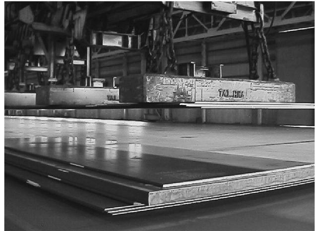
Fig. 9. Lifting the plates about 30 cm above the stack.
